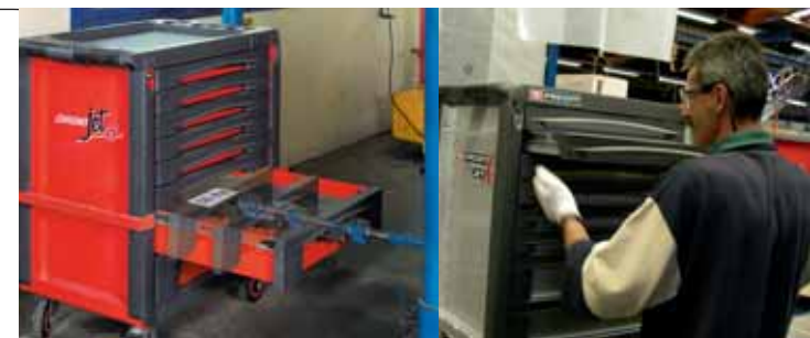
The drawers are tested over 50,000 opening / closing cycles, i.e. 10 years of use.
