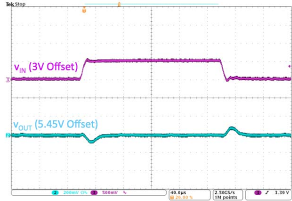
Figure 10. Line Transient, 3.0 V \leftrightarrow 3.5 V, 10 \mu\text{s} Edge, 550 mA Load
