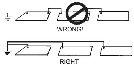
Figure 3. ESD working surface should never be grounded in series, i.e. daisy chained.
