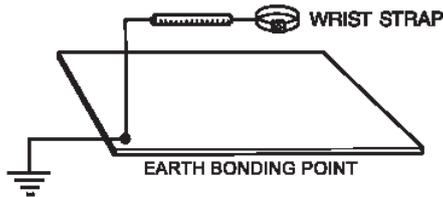
Figure 4. Earth bonding point for each workstation.
