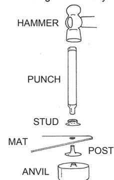
Figure 10. Using the [230660](#) Punch and Anvil.
