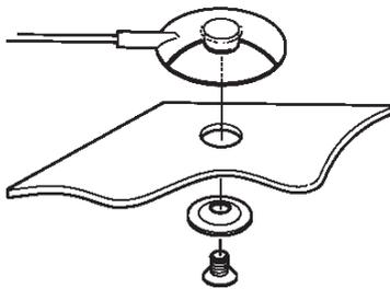
Figure 12. Installing [231280](#) to mat using supplied hardware.
