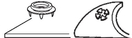
Figure 9. Installing push and clinch mat grounding snap.
