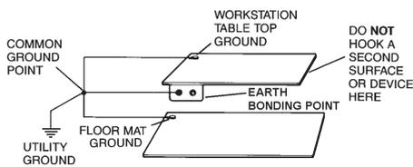
Figure 11. Earth bonding point installation.
