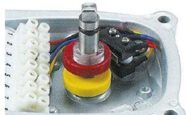
7. Now the cover can be replaced, ensure the beacon is correctly aligned and that the sealing 'O' ring is correctly fitted then securely tighten the four cover bolts.
