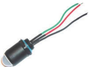
2 colour LED (3 wires) Steady Red and Steady Green. Fits to conduit entry of most switches and provides option for LED indication based upon switch contacts. The dome shaped LED is visible from narrow angles. Available voltages 24Vdc, 110Vac or 230Vac and either M20 or 1/2" NPT conduit thread. PVC conductors, fully encapsulated IP67. Maximum temperature: 60C. Housing material is polyester.
