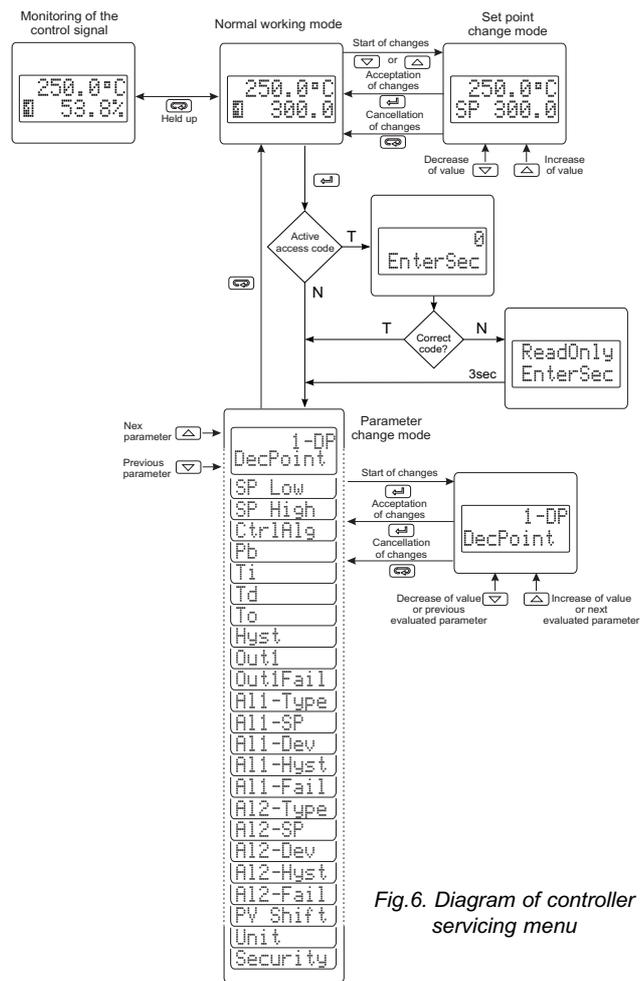
Fig.6. Diagram of controller servicing menu
