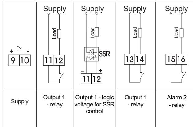
Fig.4. Connection of the supply and load circuit
