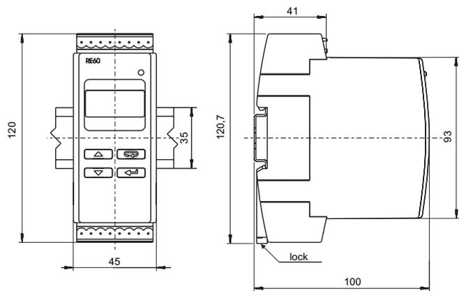
*Fig.1. Dimensions and fixing way of the controller*
