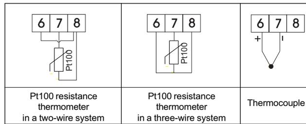
Fig.3. Connection of input signals
