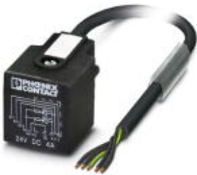
Sensor/Actuator cable, 5-position, PUR halogen-free, Black RAL 9005, free cable end, on Valve connector AD (pressure switch), with 2 LEDs, Cable length: 1.5 m
