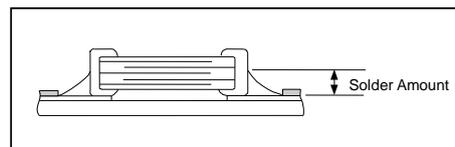
3-2. A soldering iron with a tip of φ3mm or smaller should be used. It is also necessary to keep the soldering iron from touching the components during the re-work.
