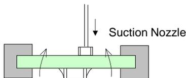
**2-2. Inserting Components with leads into Boards**
