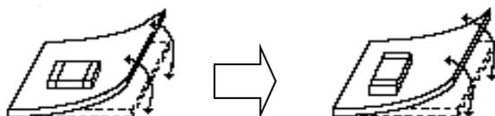
[Chip Mounting Close to Board Separation Point]
