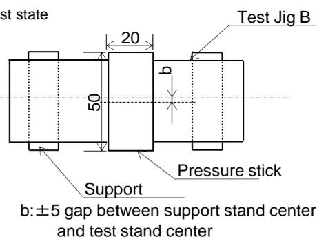
b: ±5 gap between support stand center and test stand center
