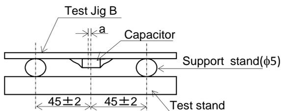
a: ±2 gap between support stand center and test stand
