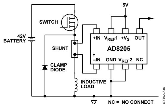
Figure 20. High-Side Switch
