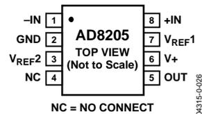
Figure 3. Pin Configuration
