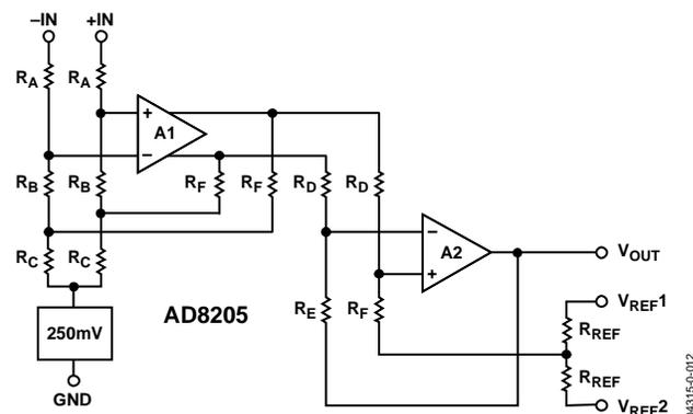
Figure 13. Simplified Schematic
