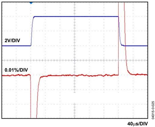
Figure 11. Settling Time
