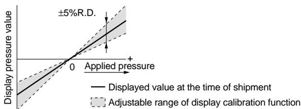
Note) When the precision indicator setting function is used, the set (differential) pressure value may change  $\pm 1$  digit.
