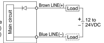
\* Install the load either on the LINE (+) or LINE (-) side.
