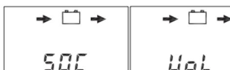
Only fixed voltage thresholds are used and the SOC bar display is faded out in all windows during voltage-guided control (UoL).
