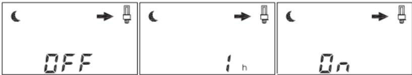
This function controls the load output only when it is dark (at night). During daylight the consumer output remains off. The connected solar module records information on the light intensity.
