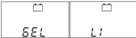
The standard setting is "Li". The setting of the battery type influences the cutoff voltage of the controller. If you use a Gel or AGM battery, you have to change the battery type to GEL.
