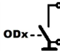
As you can see from the diagram there is no power available at the output. For an open drain output to work, the user must provide an external power source. The open drain output does nothing more than provide a path with a very low resistance to ground when it is switched on.
