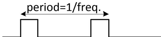
The frequency must be between 10Hz and 30 KHz. If you change the brushed frequency the program will set the corresponding duty cycle for you. You can change the duty cycle whilst the motor is running.
