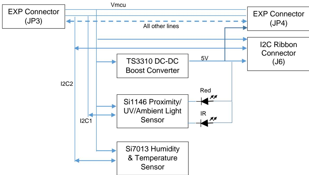
Figure 12. Biometric-EXP Block Diagram
