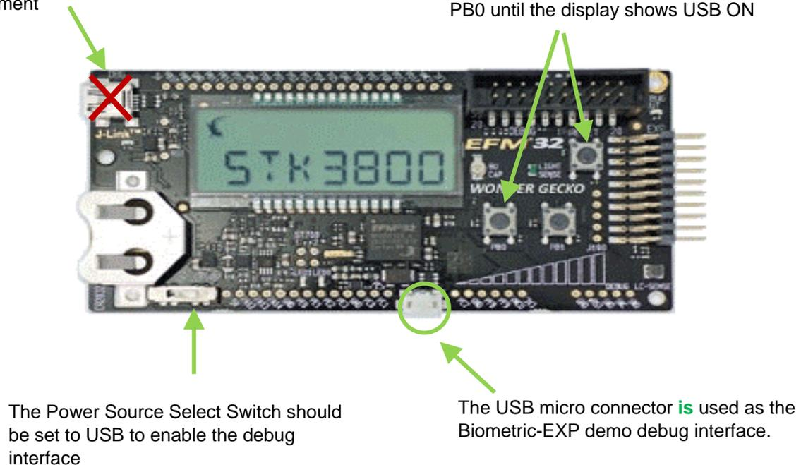
**Figure 8. Enabling and Connecting to USB Debug Mode**
