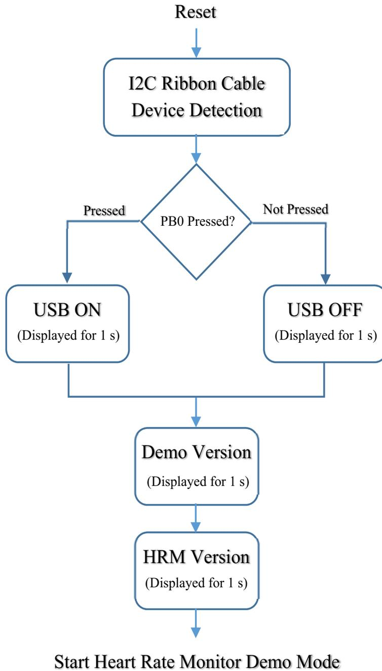
Figure 5. Biometric-EXP Demo Startup Sequence Flash Programmer Dialog
