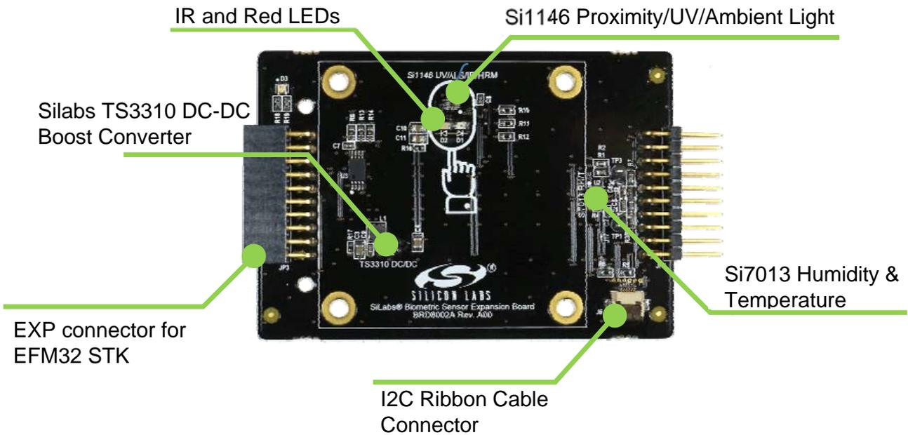
Figure 13. Biometric-EXP Hardware Component Layout
