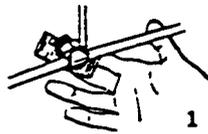
For a 25mm connector, cut a 50mm piece of Scotchfil putty and place in position.
