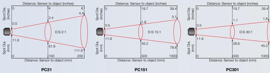
All PyroCouple sensors are fitted with precision Germanium lenses for accurate optics. Model PC21 has 2:1 optics making it suitable for most applications where the sensor can be mounted close to the target. Model PC151 is designed for small or distant targets and has an optical resolution of 15:1. Model PC301 is designed for very small or distant targets and has an optical resolution of 30:1.
