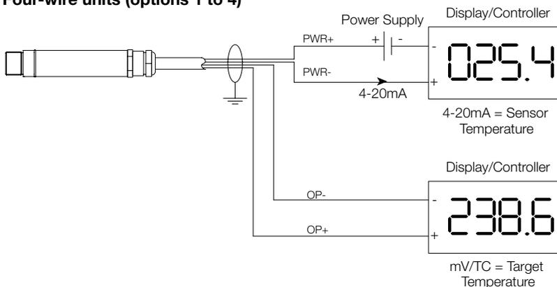
The PyroCouple Series is a range of high quality, low cost, compact sensors which measure the temperature of inaccessible or moving objects and materials. They measure temperatures from -20°C to 500°C, accurately and consistently, with an outstanding response time of 240 ms.
